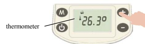
A lock child protection could be set. Press at the same time plus and minus buttons and hold about 3 seconds to lock the keyboard. A small lock icon will displayed on.
