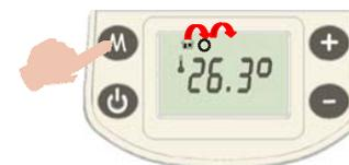
The set temperature can be adjusted using plus and minus buttons. The blinking thermometer icon indicates the setting mode.
