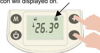
Press the two buttons at the same time for 3 seconds, again, to unlock the keyboard.
